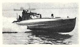
Capable of giving chase to full size destroyers this "Whippet" torpedo boat measures only 55 feet in length. Fully loaded it has maximum speed of 40 knots; cruising range of 800 miles.
