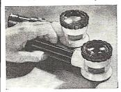
A five-power magnifying instrument combined with a flashlight, provides an illuminated two-inch field ready for instant use. A spacer ring keeps the lenses in focus, and the light is so di-rected that while it illuminates object being inspected, it does not strike eyes.
