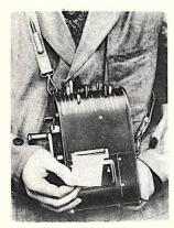
Tickets and transfers can be printed as needed by this German device. This eliminates punching.
