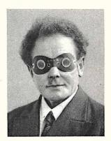
These novel spectacles can be used instead of a microscope. They obtain their microscopic power from specially-processed dark
