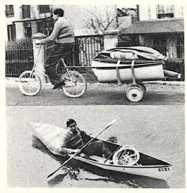
After designing a collapsible bicycle for land travel, French inventor, Louvet, shown above, set to work on a folding craft for water travel. A small trailer hauls folded canoe overland.
