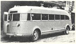
Featuring a body constructed of aluminum instead of the usual steel, this modern bus reduces gross weight by two tons. A V-8 Ford motor is sufficient to power the new motor coach.
