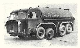
Used to haul oil to the Persian Gulf from fields 400 miles away, this 8-wheeled, 3,700-gallon tanker crosses a mountain pass 8,000 feet high. All 8 wheels can be braked at once.
