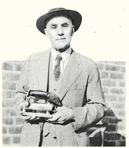
This iron is partly filled with water which is heated by the same electricity that heats the iron. The clothes are steam moistened from the bottom of the iron as the ironing goes on.
